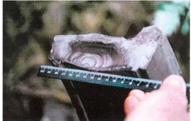
Figure 7: The failed tyre that caused the derailment
