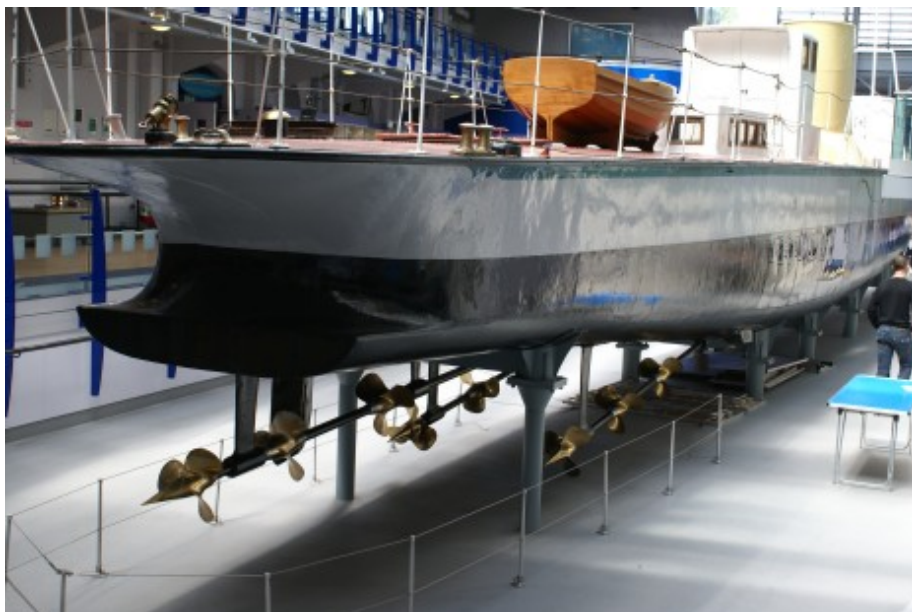
Figure 2: Turbinia's array of propellers
