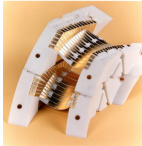
Figure 3: Thin film heat transfer gauges: early Macor blade (left), later 3-D blade (right)
