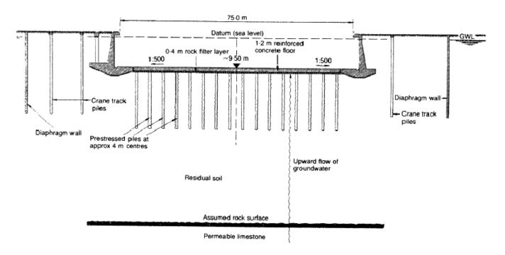
Figure 1: Typical cross-section of new No. 5 dry dock as built in 1977
