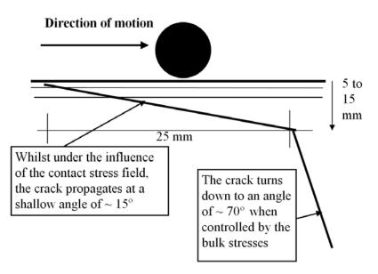
Figure 3: Crack propagation in rails
