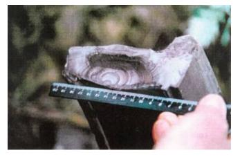
Figure 7: The failed tyre that caused the derailment
