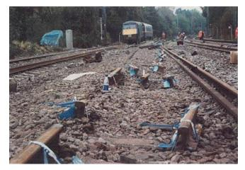
Figure 5: Broken rail at Hatfield
