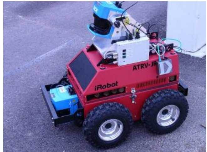
Figure 1: "Marge" — an all terrain autonomous vehicle with 2D and 3D laser scanners. Her partner, "Homer", is not shown. The cube near the front bumper is the 2D laser scanner used to build the basement map in Figure 2. The second cube is mounted on a "nodder" and allows the vehicle to scan its environment in 3D.
