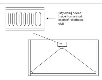
One bay of a multi-storey steel-framed building, incorporating the slit yielding device to reduce earthquake damage
